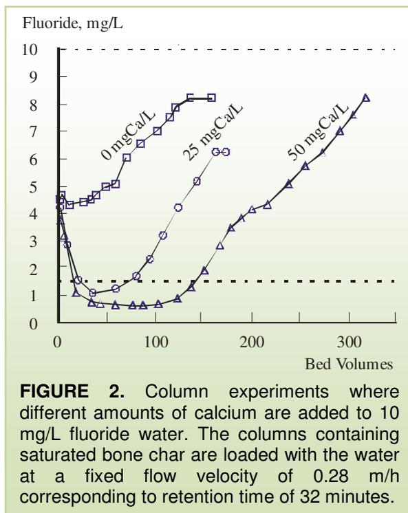
**FIGURE 2.** Column experiments where different amounts of calcium are added to 10 mg/L fluoride water. The columns containing saturated bone char are loaded with the water at a fixed flow velocity of 0.28 m/h corresponding to retention time of 32 minutes.
