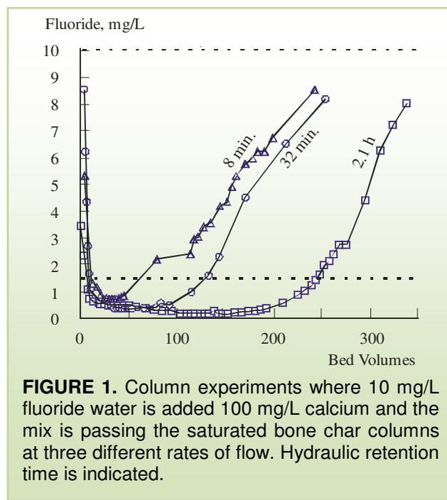
**FIGURE 1.** Column experiments where 10 mg/L fluoride water is added 100 mg/L calcium and the mix is passing the saturated bone char columns at three different rates of flow. Hydraulic retention time is indicated.
