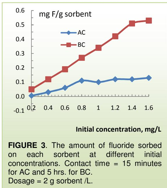
**FIGURE 3.** The amount of fluoride sorbed on each sorbent at different initial concentrations. Contact time = 15 minutes for AC and 5 hrs. for BC. Dosage = 2 g sorbent /L.
