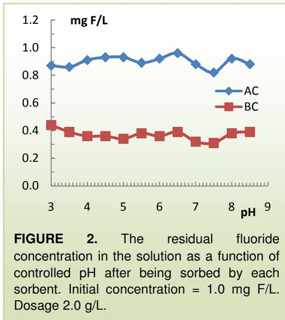
**FIGURE 2.** The residual fluoride concentration in the solution as a function of controlled pH after being sorbed by each sorbent. Initial concentration = 1.0 mg F/L. Dosage 2.0 g/L.
