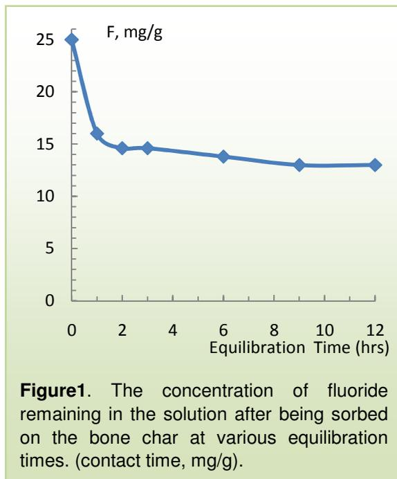
**Figure1.** The concentration of fluoride remaining in the solution after being sorbed on the bone char at various equilibration times. (contact time, mg/g).
