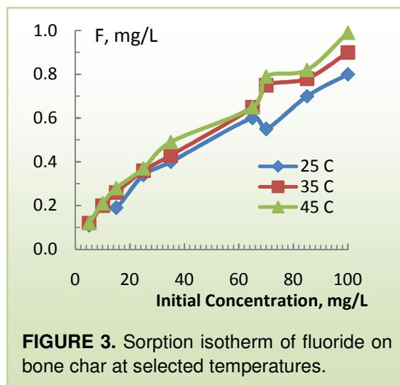
**FIGURE 3.** Sorption isotherm of fluoride on bone char at selected temperatures.
