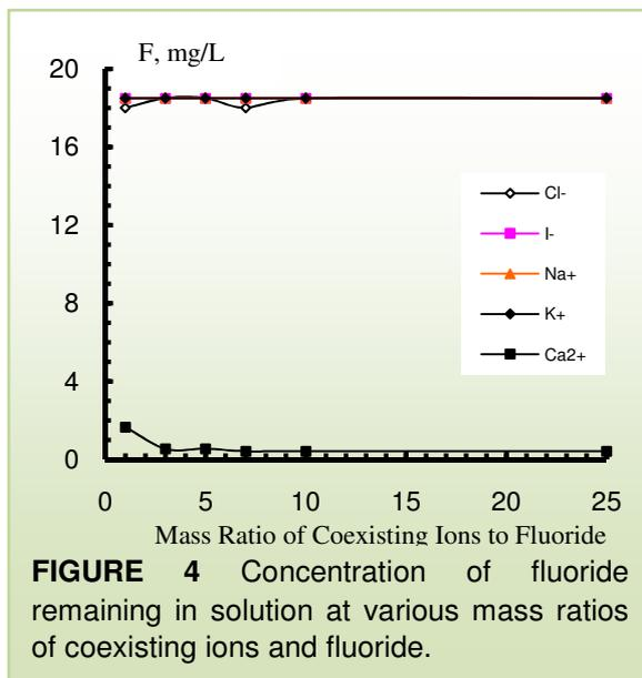
**FIGURE 4** Concentration of fluoride remaining in solution at various mass ratios of coexisting ions and fluoride.
