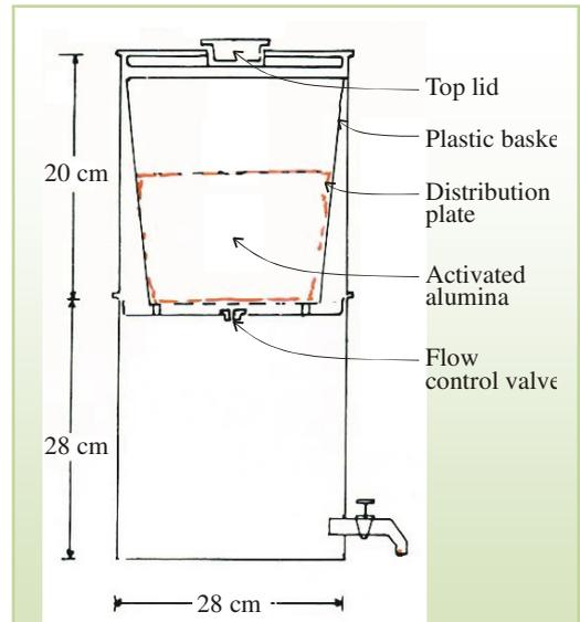
**FIGURE 2.** Sketch of the domestic filter utilising activated alumina.
