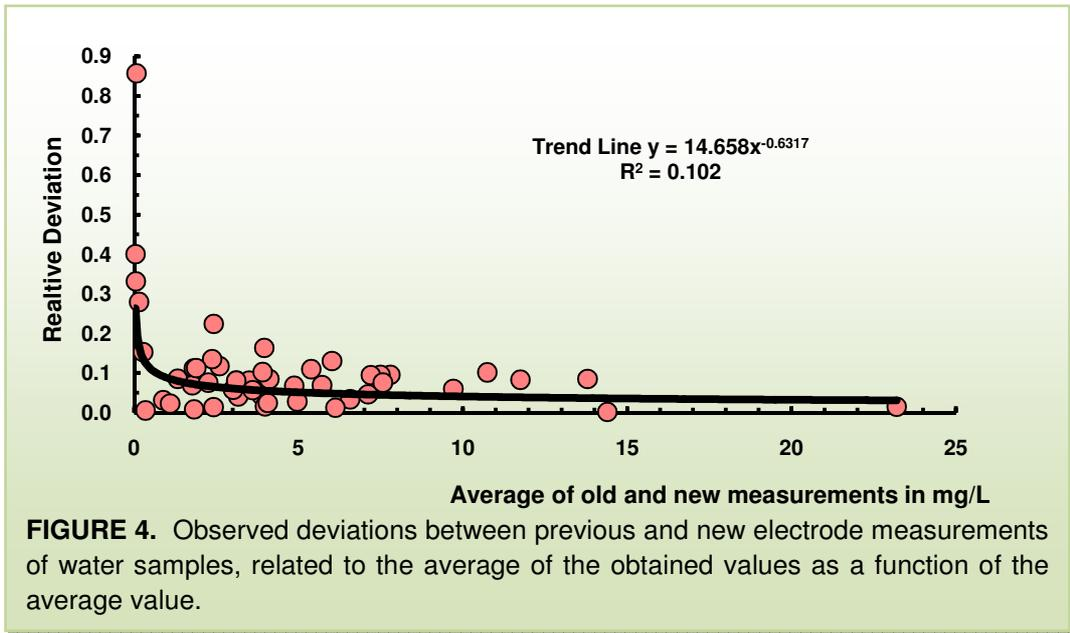
**FIGURE 4.** Observed deviations between previous and new electrode measurements of water samples, related to the average of the obtained values as a function of the average value.
