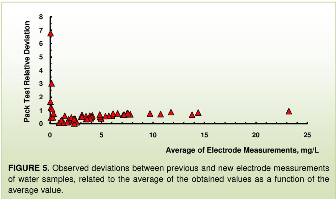
**FIGURE 5.** Observed deviations between previous and new electrode measurements of water samples, related to the average of the obtained values as a function of the average value.
