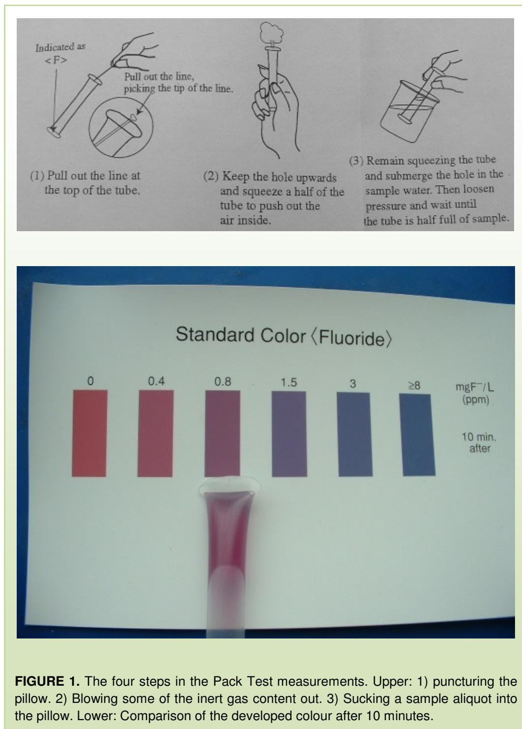
**FIGURE 1.** The four steps in the Pack Test measurements. Upper: 1) puncturing the pillow. 2) Blowing some of the inert gas content out. 3) Sucking a sample aliquot into the pillow. Lower: Comparison of the developed colour after 10 minutes.
