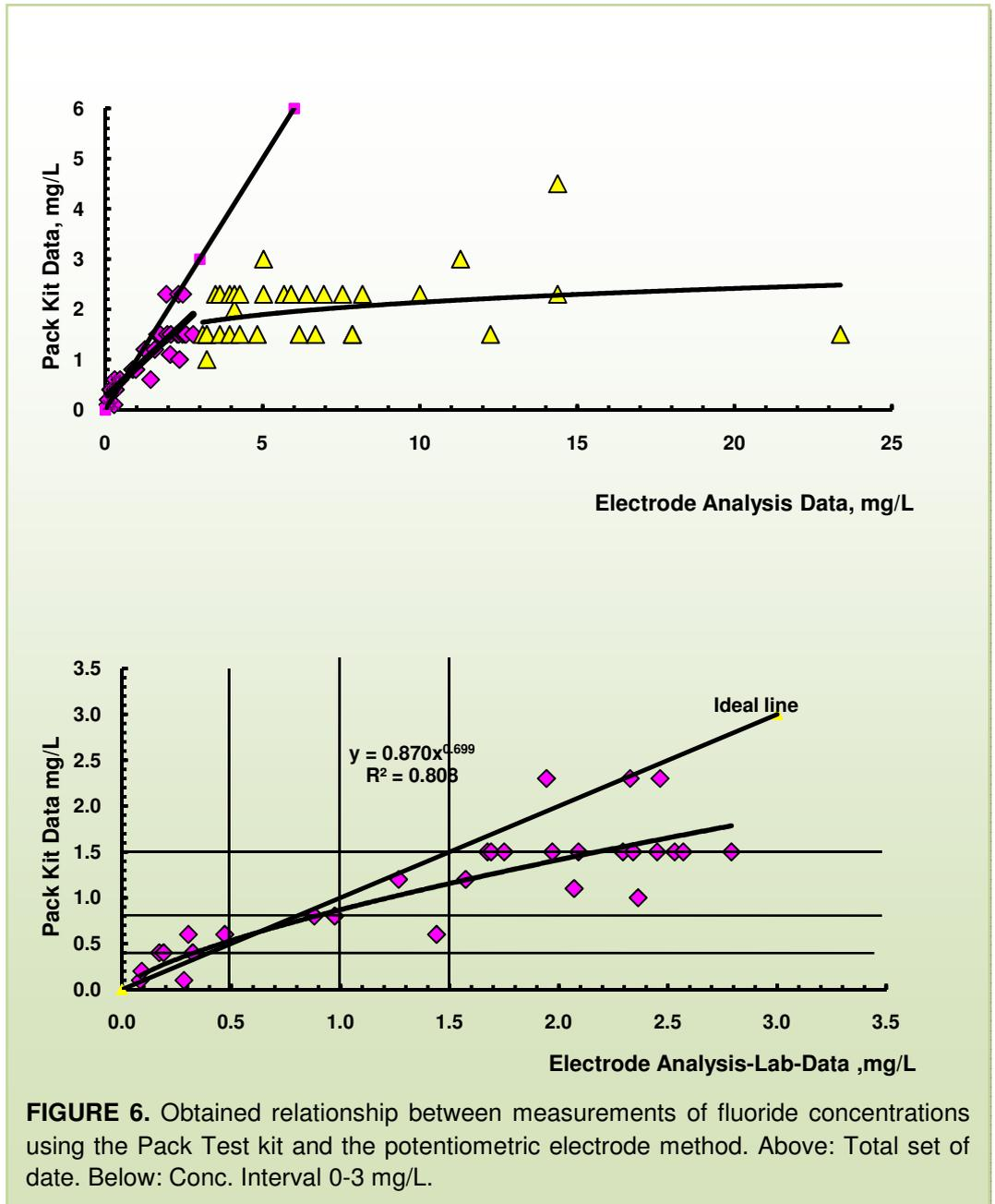
**FIGURE 6.** Obtained relationship between measurements of fluoride concentrations using the Pack Test kit and the potentiometric electrode method. Above: Total set of date. Below: Conc. Interval 0-3 mg/L.
