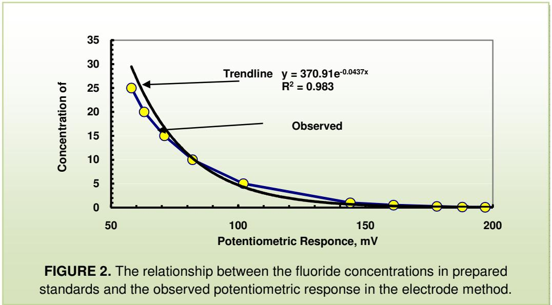
**Standard calibration curve:** An extended standard curve was prepared to cover the normal fluoride concentrations prevailing in the water of the Arusha Region. This included 0.025, 0.05, 0.10, 0.25, 0.50, 1.00, 5.00, 10.00, 15.00, 20.00 and 25.00 mgF/L. The obtained calibration curve is shown in Figure 2.
